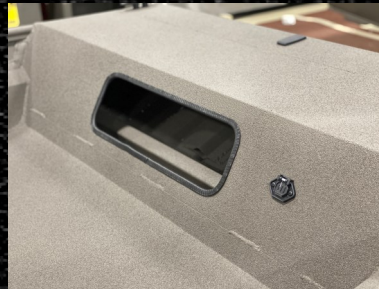
Front Deck Storage Hole
