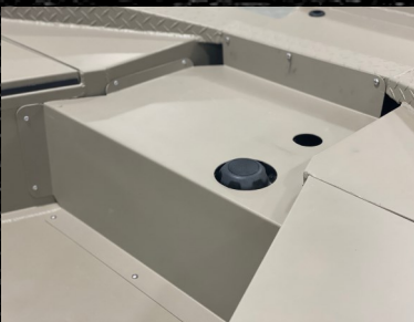
Direct Fill Fuel Tank
